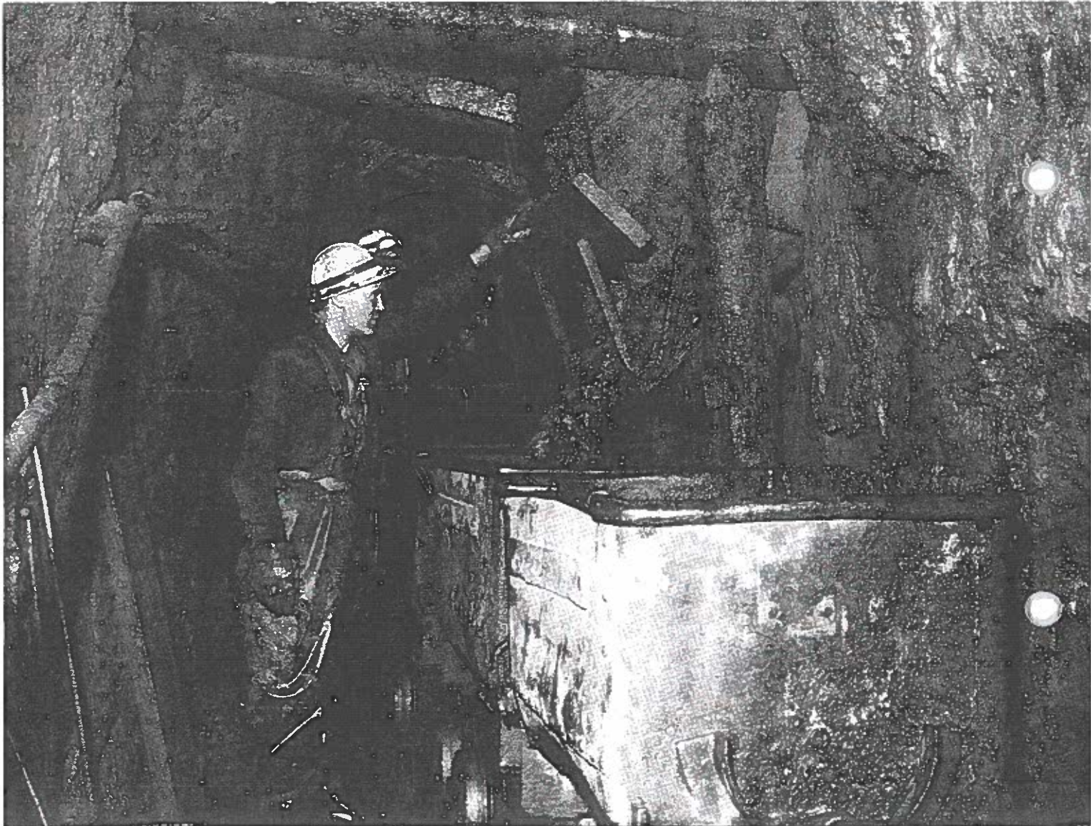
Alfred Blackett loading a tub from a hopper on the main horse level, Blackdene Mine 1964-5. Photograph - Appleby Frodingham Steel Co/Branch of United Steel Co.Ltd
