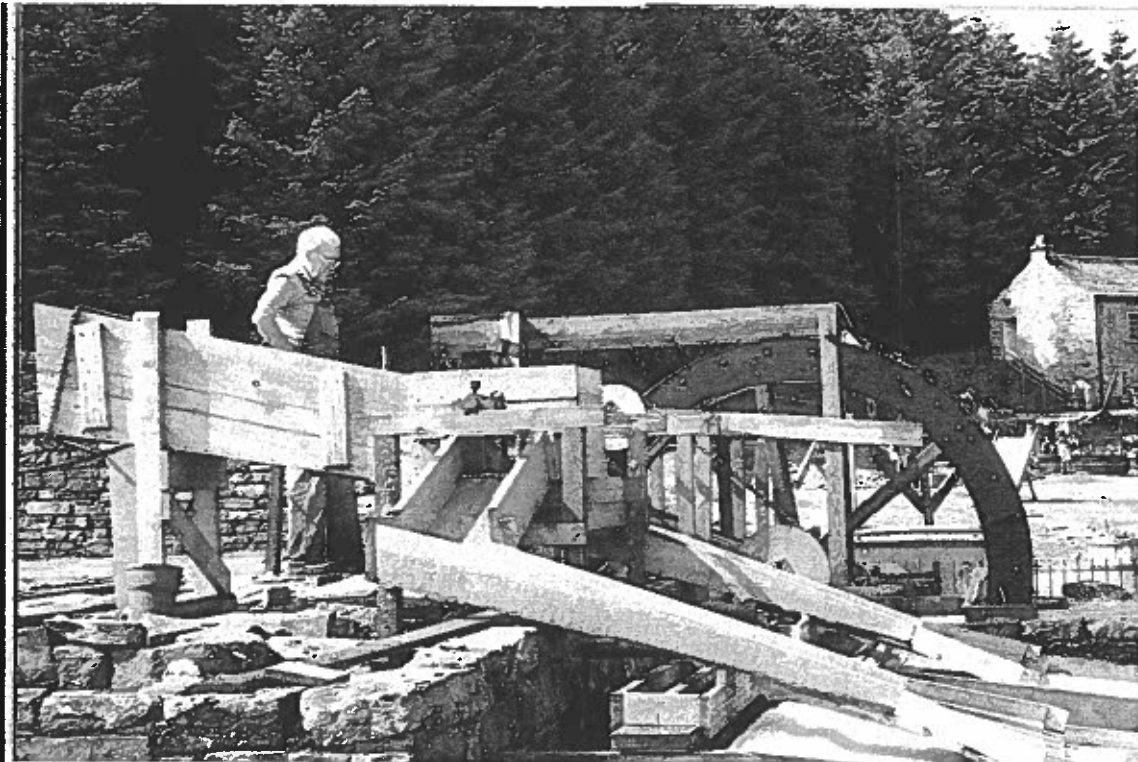
Brunton buddles under trials. A closer view showing the chain drive from the wheel.
