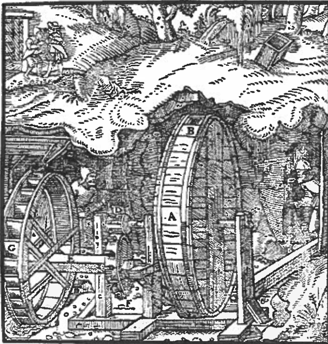
A—HOLLOW DRUM. B—ITS REDWOOD-HOLE. C—AXLE WITH FANS. D—DRUM WHICH IS MADE OF BUNDLES. E—LOWER AXLE. F—ITS TOOTHED WHEEL. G—WATER WHEEL.
